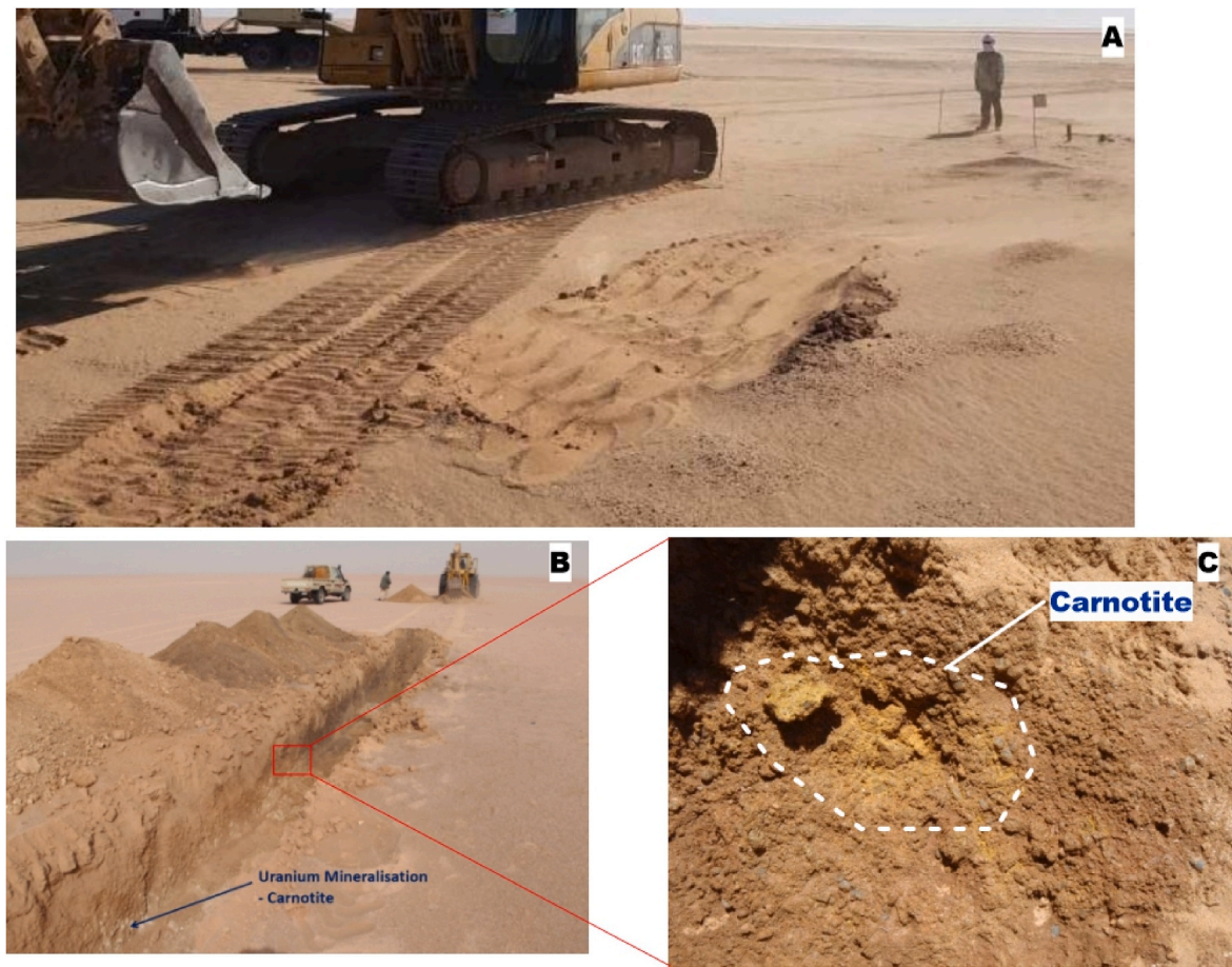
Fig. 9. Field view of calcretes U-deposit of Tiris project: A- Field appearance; B- surficial uraniferous layers; C- uranium bearing mineral (carnotite) (Aura Energy, 2022).
