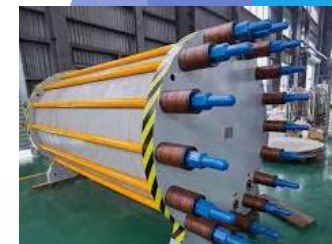
John Cockerill 5 MWe Electrolyzer
